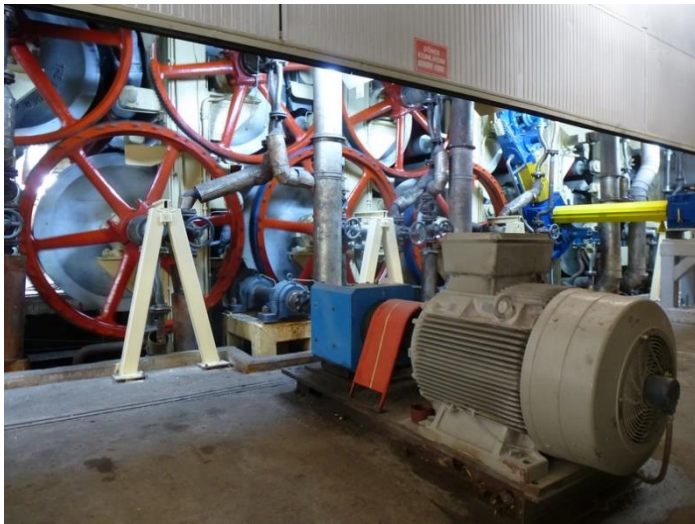
Fig. 1: the old open wheel drive (left)
