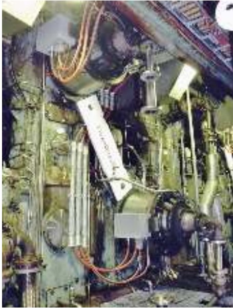
Fig. 5: 2 FlexoDirect® with steam heads on the driving side of the PM6
