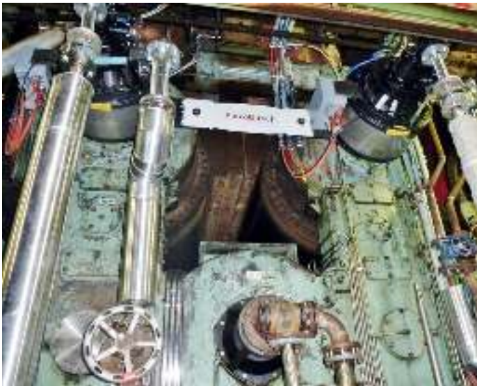
Fig. 6: 2 FlexoDirect® with torque support in horizontal connection
