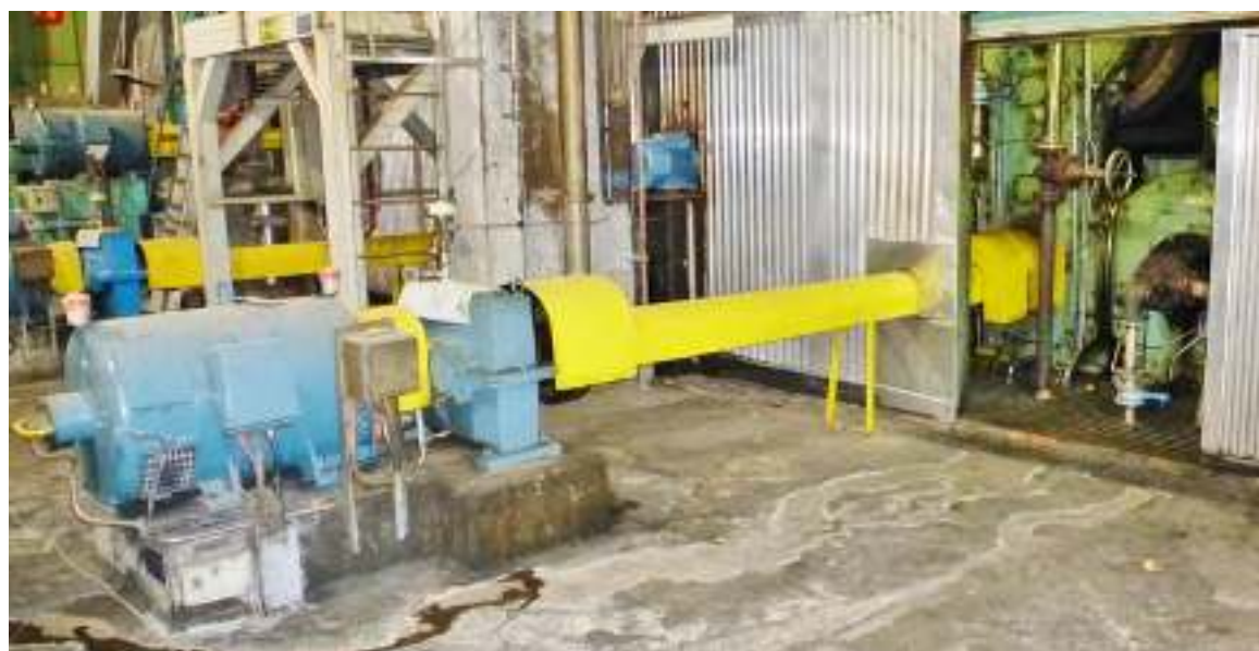
Fig. 4: Conventional drive solution with DC motor, pre gearbox and coupling, outside of the dryer hood
