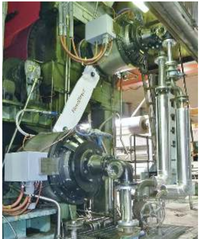
The new direct drive FlexoDirect® in permanent magnet technology
