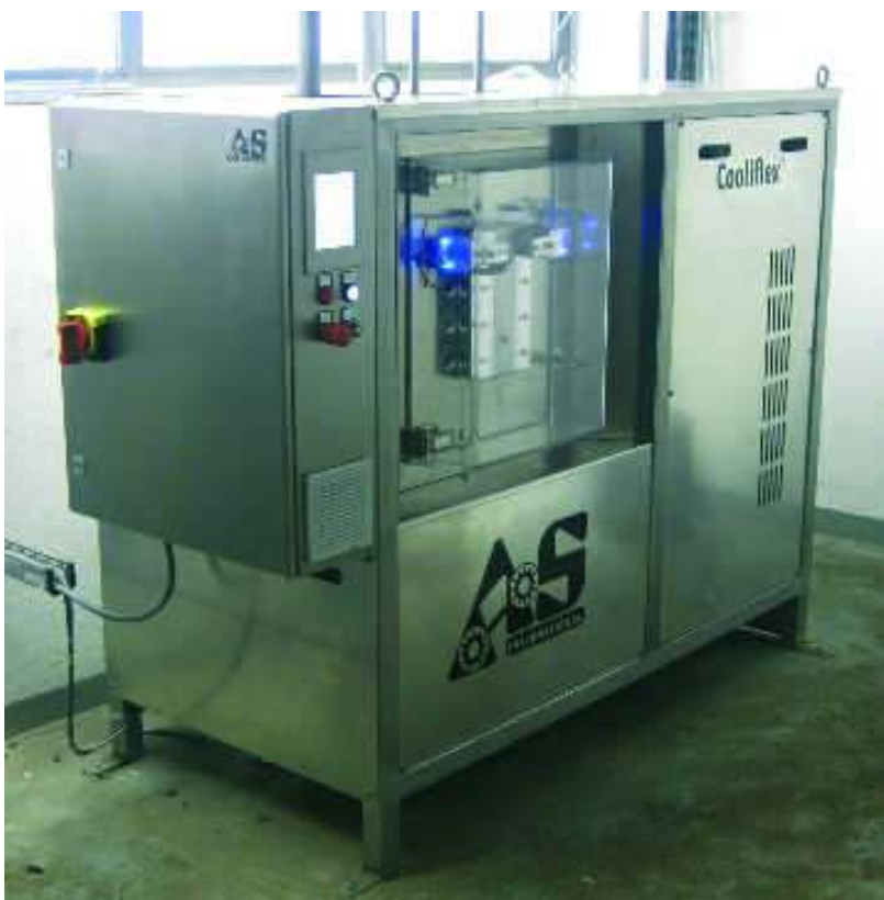
Fig. 5: The cooling and heating aggregate Cooliflex®
