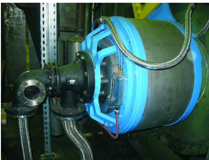
Fig. 4: The FlexoDirect and steam head
