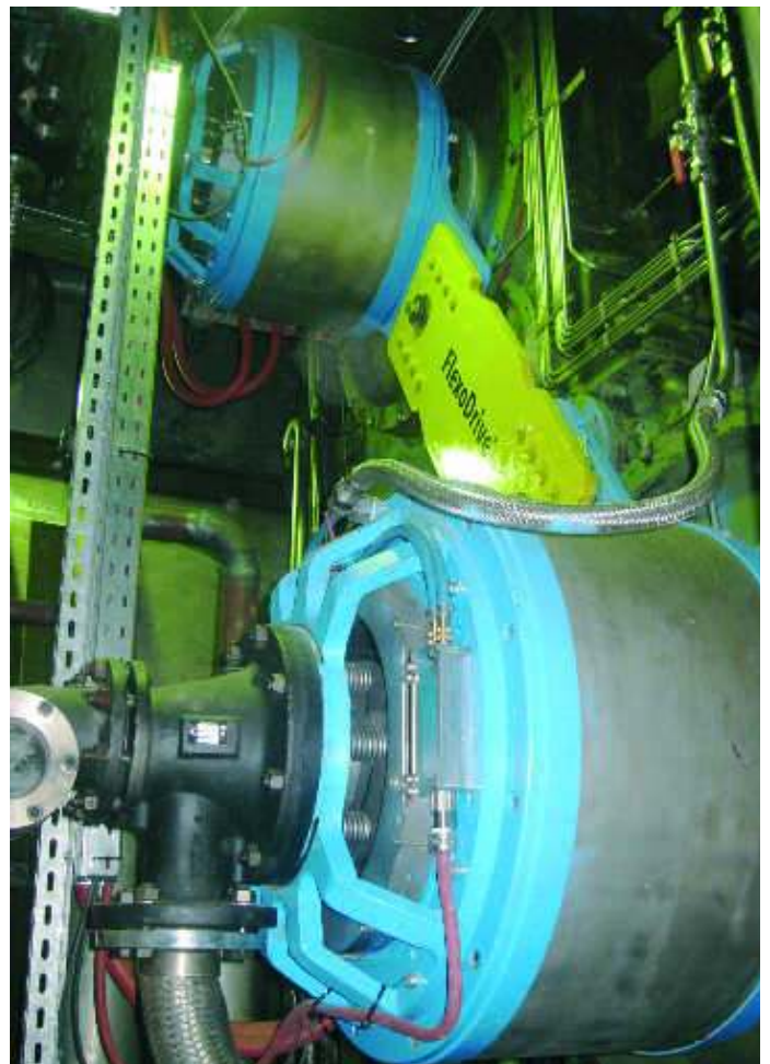
Fig. 8: Coupling of two FlexoDirect via patented torque support
